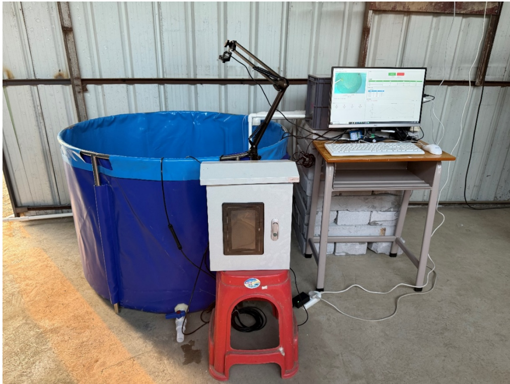
Figure 4. An experimental aquaculture setup was used to collect data, including a stainless-steel tank with an underwater HD camera, infrared lighting, and a water-quality probe connected to a data acquisition unit.
